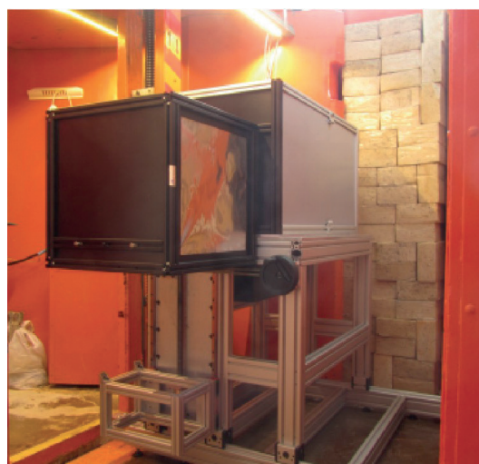
Figure 1. a) The 3D view of the facility. b) The light-tight optical assembly, ImageFrame hosting the scintillators, the mirror, the optics and the camera
