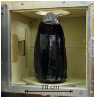
Fig. 1. An obsidian core in the sample holder of the Budapest NIPS-NORMA station
