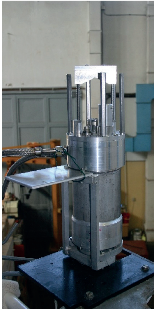
◀ Figure 2. Assembled Bagira4 head with gas and electrical connectors
