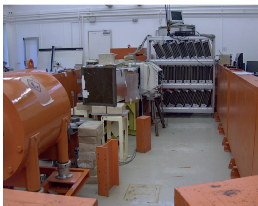
Figure 3. The time-of-flight neutron diffractometer (ToF-ND) at the thermal neutron beam-line No.1, with the new large area back-scattering detector bank.
