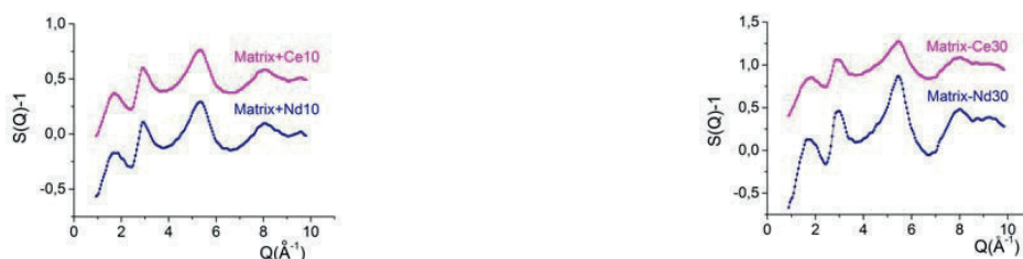
Figure 1. Neutron diffraction total structure factors for Matrix-Nd10(30) (blue) and Matrix-Ce10(30) (magenta) glasses and RMC fits (solid line).
