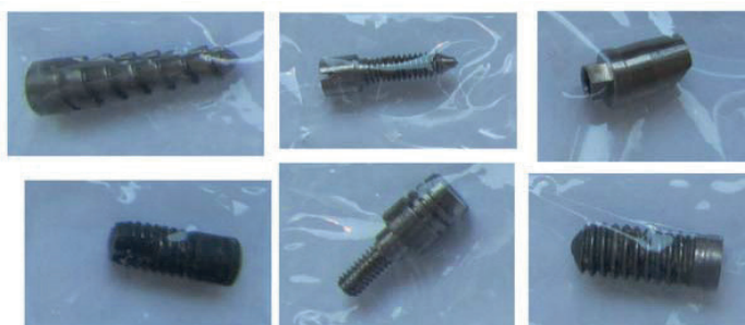
Fig. 1 Titanium implants sealed in Teflon bags for the PGAA measurements.
