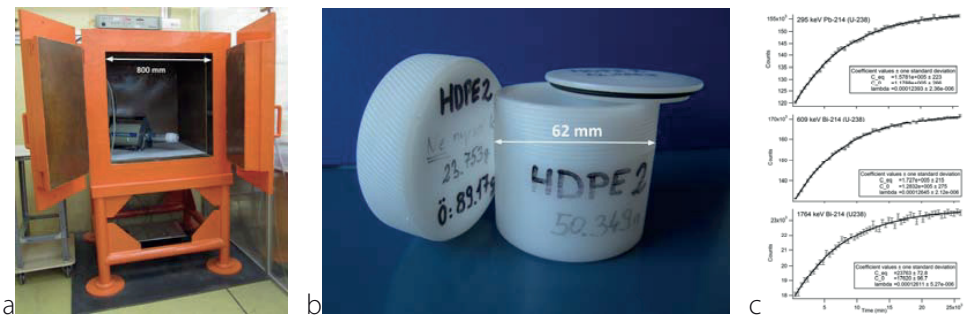
Fig. 1. (a) Photo of the low-background counting chamber (DÖME); (b) a special sample container made of HDPE; (c) saturation curves for the activity concentration in a sealed container.
