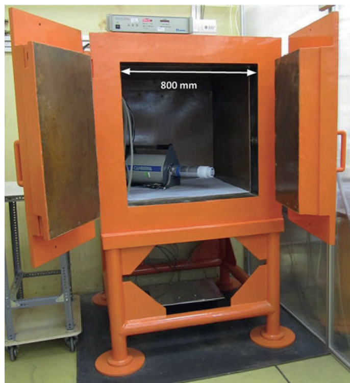
Figure 2. The iron chamber of the DÖME counting station.
