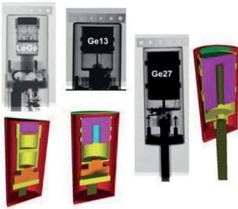
Fig.1. the X-ray image and geant4 implementation of the three HPGe detectors
