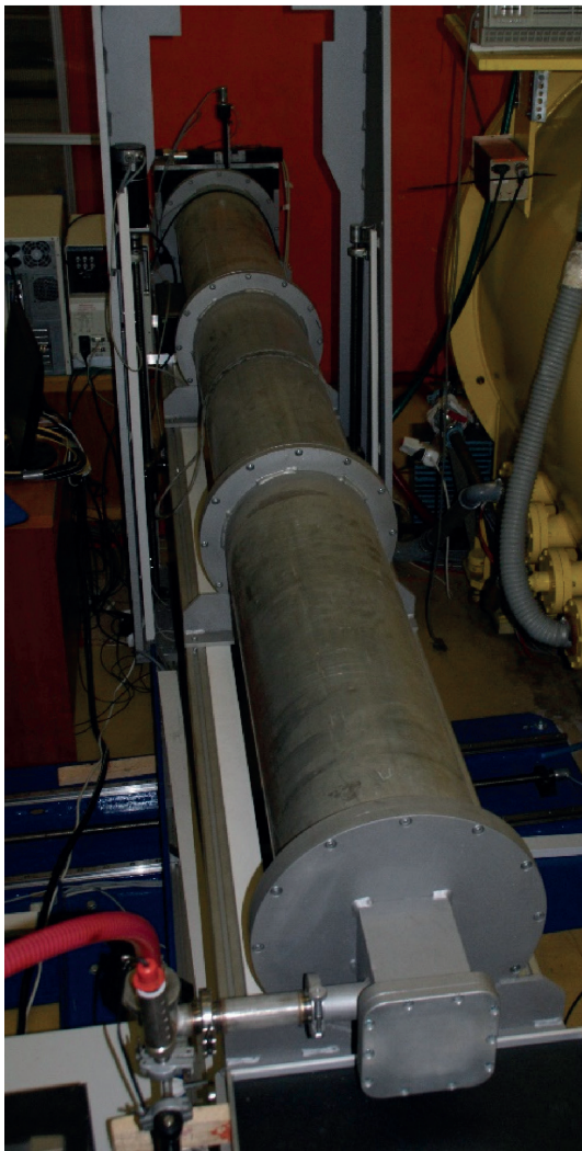
◀ Figure 1. Post sample flight tube and detector positioning mechanism of the FSANS diffractometer.
