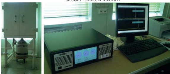
Fig. 2. the new counting station D3 with the ORTEC DSPEC 502 digital gamma spectrometer
