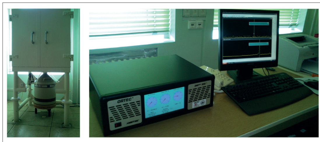
Figure 1. ▶ The "D5" gamma spectrometer of the NAA laboratory
