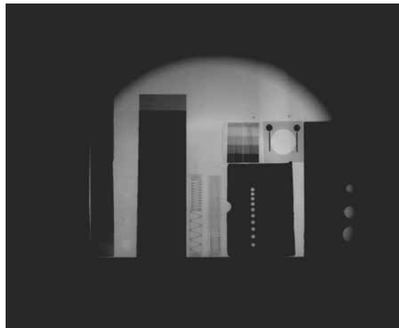
Fig. 2. NR picture of the two springs after the heat-treatment
