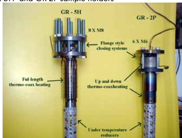
Figure 1. Flange style closing system on GR-5H and GR-2P sample holders
