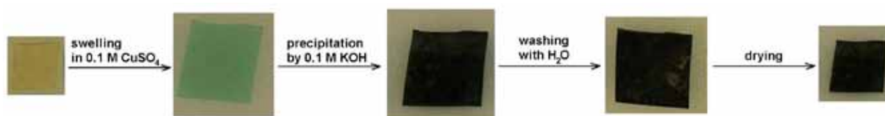
Figure 1. Illustration of the preparation procedure on the network EPI filled with CuO particles.
