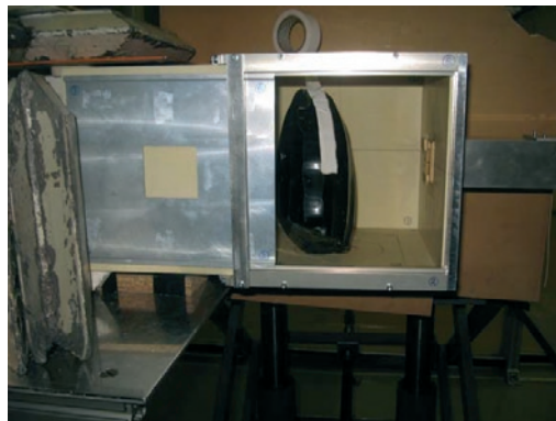
Figure: Measurement of large obsidian core at the NIPS/NORMA station
