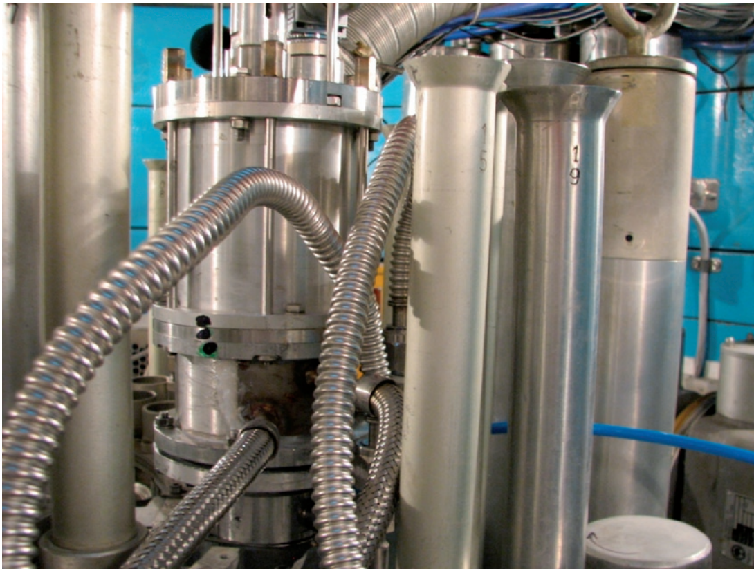
◀ Figure 2. Assembled Bagira3 in the reactor channel with the view of the rotating engine
