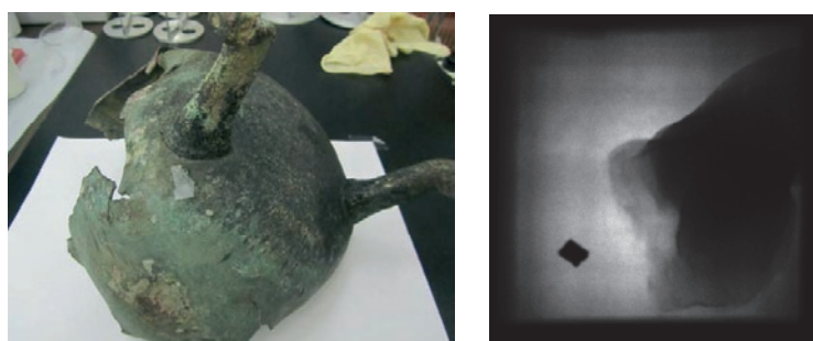
Figure 1: a, Photo of a cauldron with Gd marker; b, Neutron radiography of one of the cauldron's legs with the Gd marker
