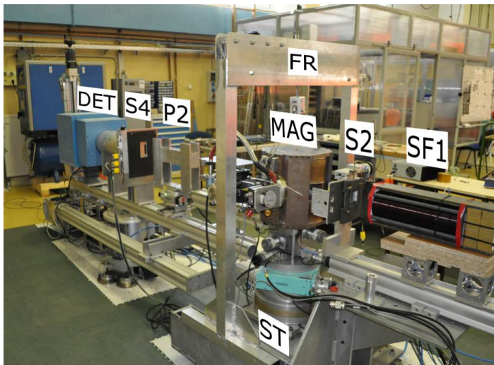
Figure 2 Partial view of the GINA reflectometer. Components are made as explained in Figure 1 apart from the sample environment with the electromagnet (MAG) with mounted closed-cycle cryostat. The magnet weight is partially relieved by
