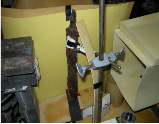
Fig. 1 PGAA setup for iron sword
