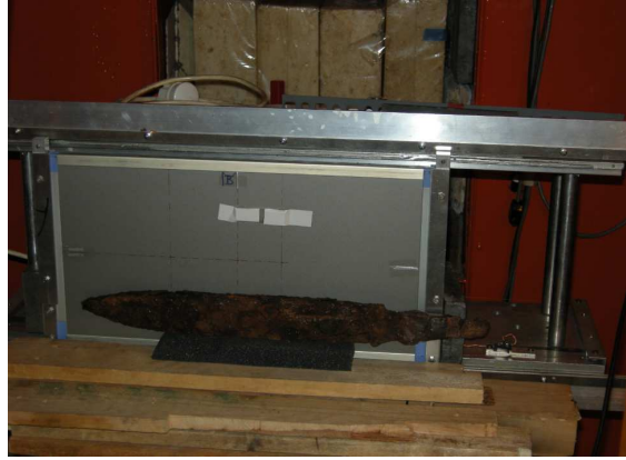
Fig. 2 X-ray radiography setup for iron sword
