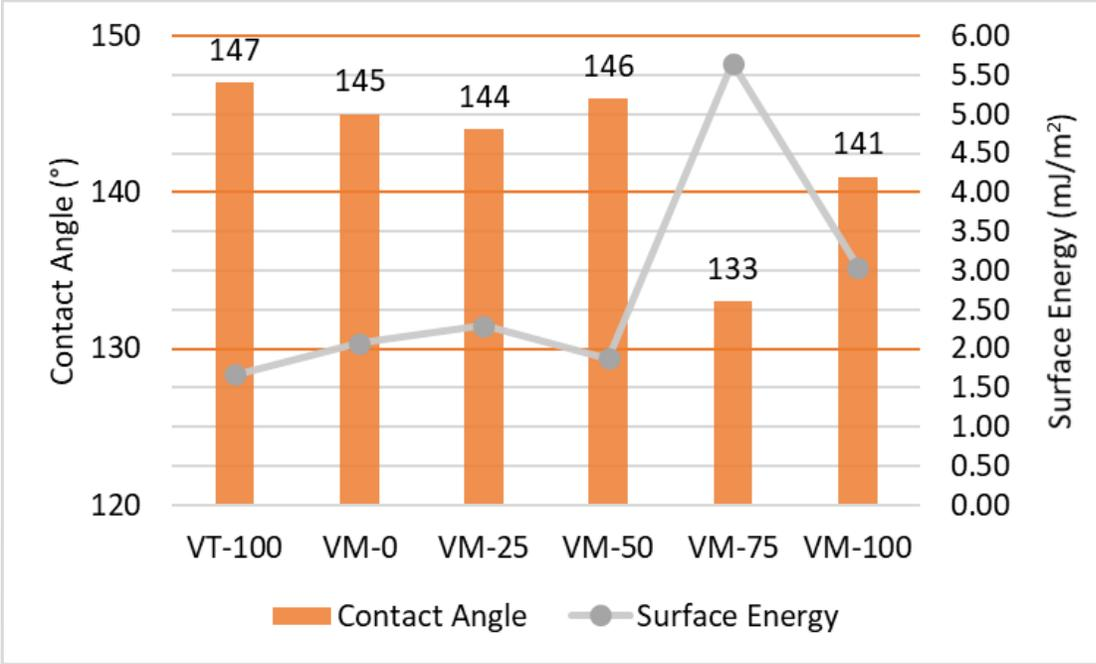
Hydrophobic behaviour of the samples in VT series
