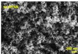
distinct and uniformly distributed pores and fine silica particles
