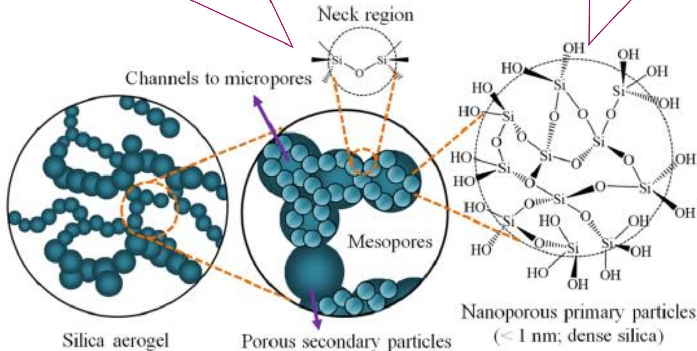
Silica xerogels prepared with conventional tetraalkoxysilanes such as tetraethylorthosilicate (TEOS), tetramethylorthosilicate (TMOS) are rich in surface silanol groups (Si-OH) which are the main source of hydrophilicity.
