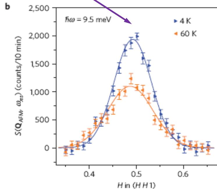
Spin excitations in the vicinity of the AFM wavevector  $\mathbf{Q}_{\text{AFM}}$ , in the superconducting ( $T = 4 \text{ K}$ ) and the normal state ( $T = 60 \text{ K}$ ).
