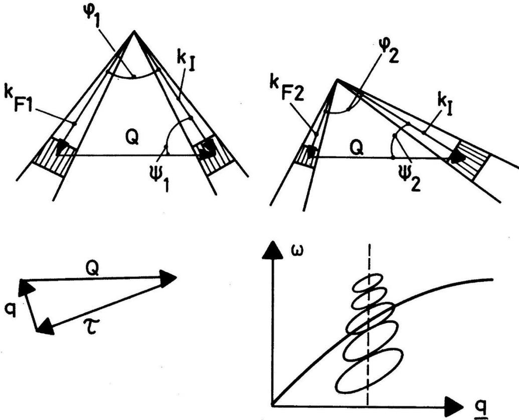
Fig. 4. Q-constant scan with  $k_I$  fixed.  $\varphi$  and  $\psi$  are scattering angle and sample orientation. The hatched areas give the distributions of  $k_j$  around  $k_I$  and of  $k_f$  around  $k_F$ .  $g$  is the phonon wavevector. In  $g$ - $\omega$  space a constant  $Q$  scan is drawn with varying resolution. (DORNER, 1976)
