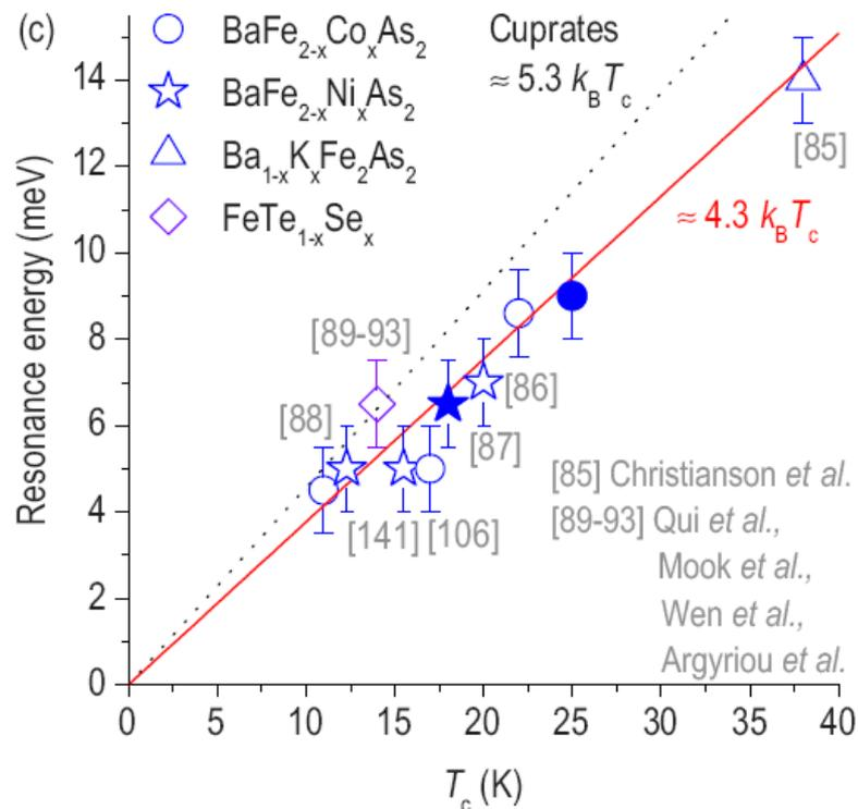
Resonance energy vs  $T_c$  for different Fe-based superconductors.
