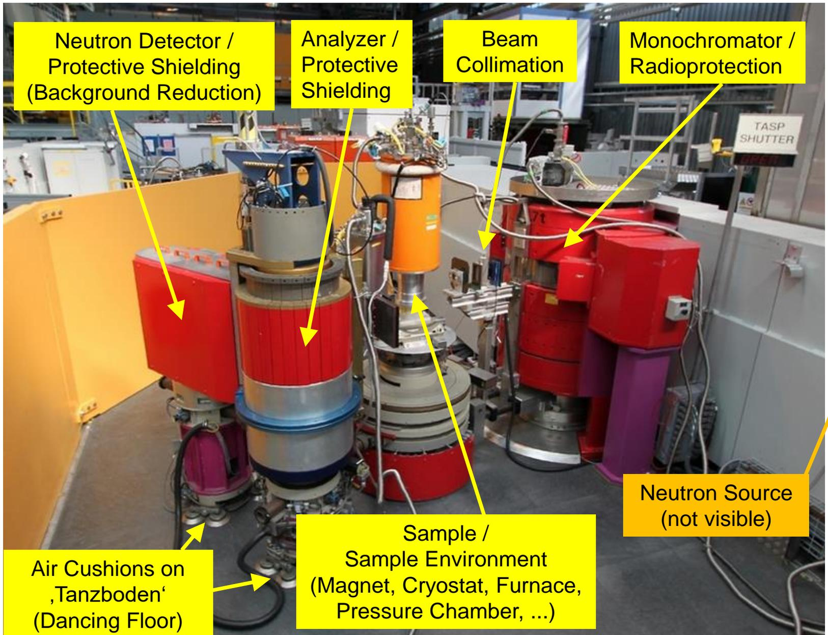
Three Axes Spectrometer TASP / SINQ
