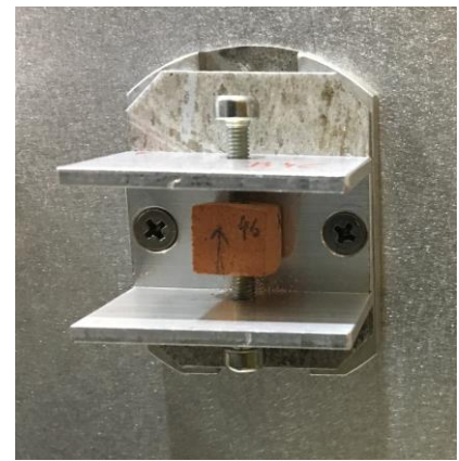
Cubic sample mounted in sample holder in F-view. Orientation sample and relative direction of beam recorded
