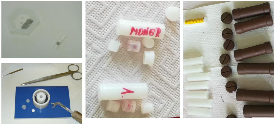
Figure 3. Few mg of powdered samples are wrapped in Whatmann 41 filter paper which is hydraulically pressed for pellet and placed into high purity polyethylene capsules. Larger polyethylene carrier is loaded into VESPEL plastic, ready for irradiation.
