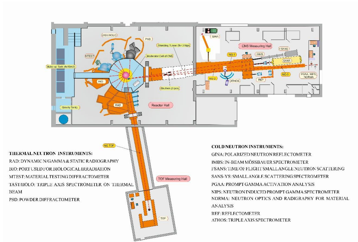
Figure 10. Layout of the horizontal neutron beam facilities at the Budapest Research Reactor
