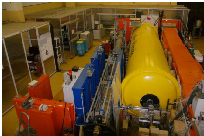
Figure 5. Image of the detector tank and sample environment of Yellow Submarine
