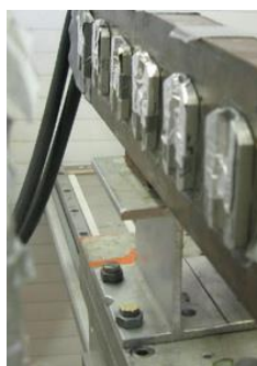
Figure 9. 6 position sample holder with temperature regulation
