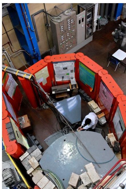
Figure 1. a) Schematic view and b) photo of the PSD neutron diffractometer
